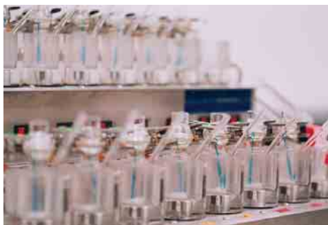
In vitro percutaneous absorption system containing Franz static diffusion cells and drive console.
