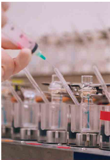
Sampling of receptor solution for assay from an in vitro percutaneous absorption system using Franz static diffusion cells.
